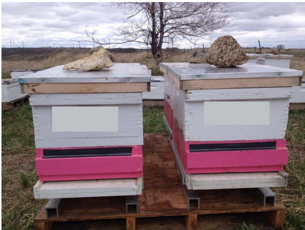
Figure 2. Arrangement of colony monitoring devices. Each colony was fitted with both a pollen trap (pink, above bottom board) and scale (below bottom board). Photo: Clint Otto, USGS-NPWR.
